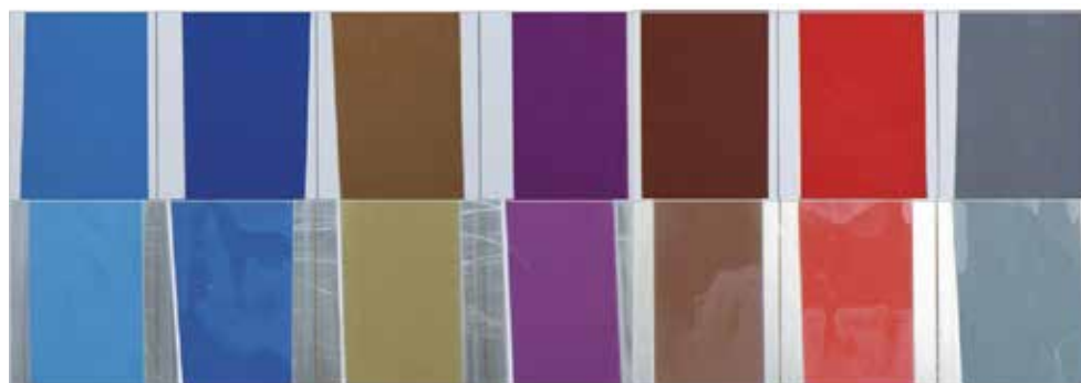
Photo illustration of UV-test, method ISO4892-2 in an Atlas Suntest XLS+ with Xenon Arc lamp.
